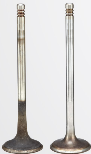
Works to remove carbon build up from intake valves
